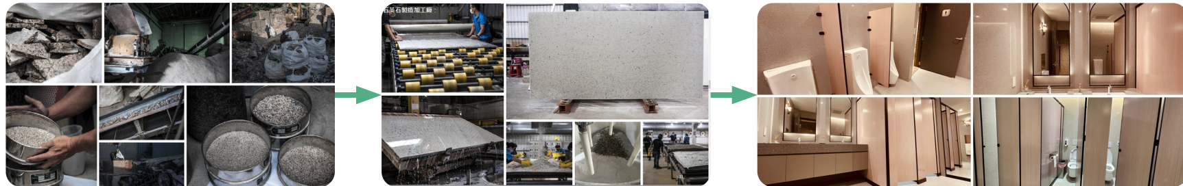
▲ Most of the old stones removed from the old workplace are too broken to be used directly. Through crushing, selecting, pressing and cleaning, we can recreate large pieces of stone that can be used in large quantities for interior decoration.
